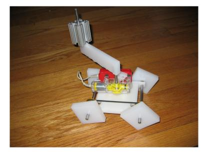
A three wheel version is also possible, and the wheels would be  $30^{\circ}$  out of phase, replacing the  $22.5^{\circ}$  for the four wheel version. Versions with more than 4 wheels are also possible, and might be advantageous in smoothing the motion of the vehicle.
