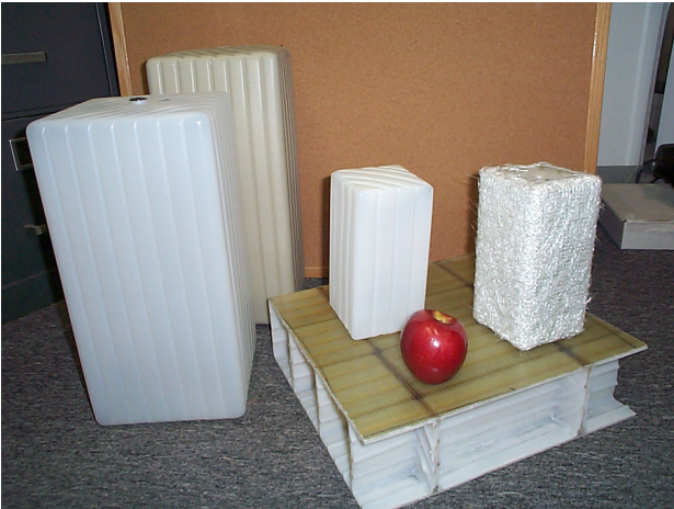
Figure - 2, Large segment 8"x 8" x 16", small segment 4"x 4"x8", segment wrapped with fiberglass fabric, and sandwich panel (bottom right).
