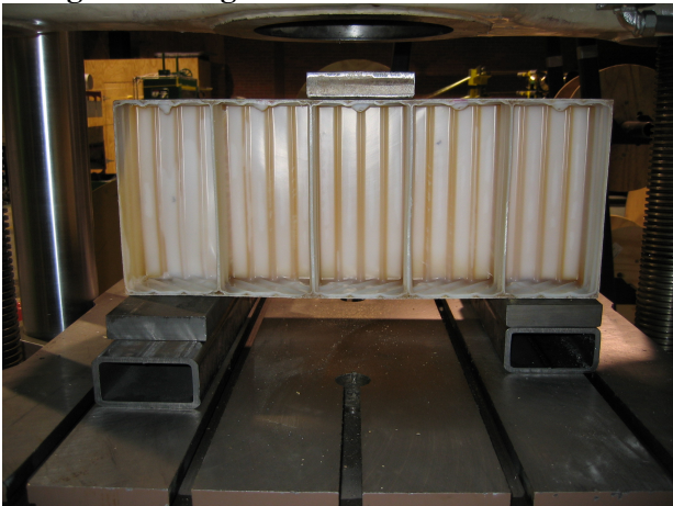
Figure - 8, Panel setup for 3-point shear test. This picture was actually after failure (Figure #9) with the load removed, the panel showed little sign of damage.
