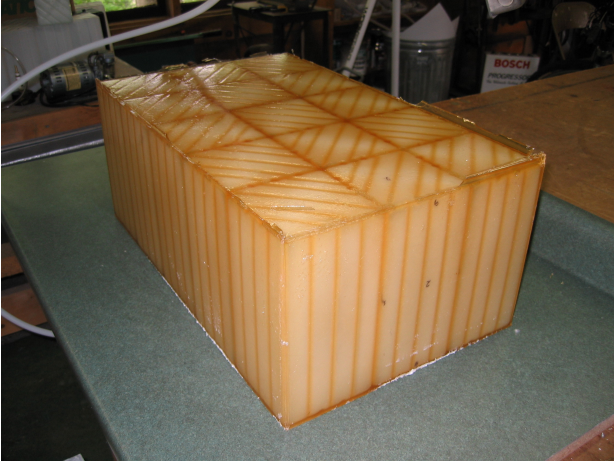
Figure - 6, As-molded panel after vacuum infusion with polyester resin (3 segments wide x 5 long).
